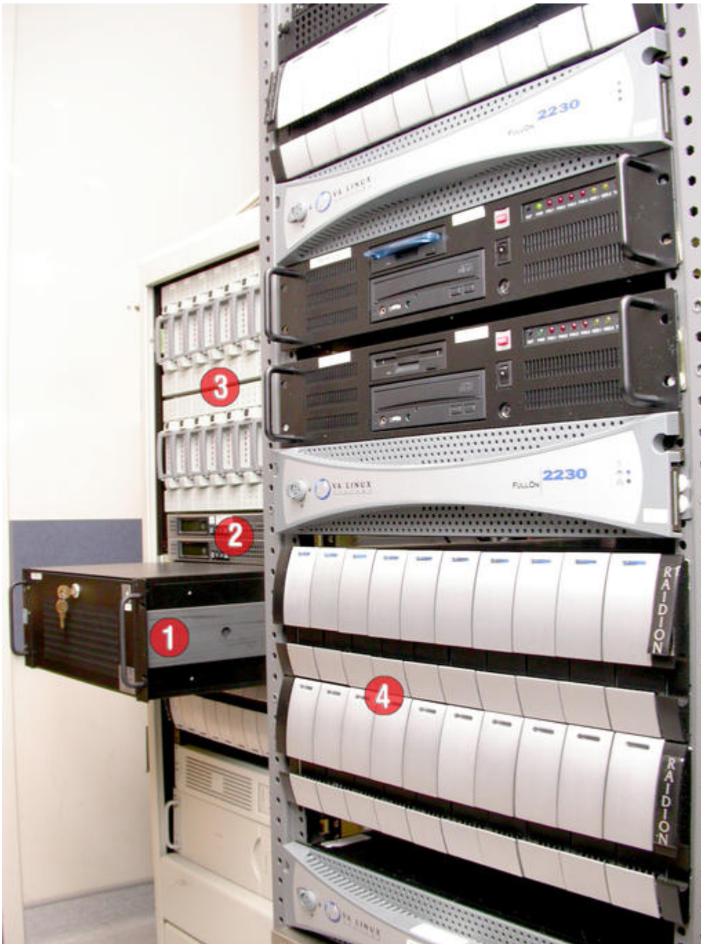
Figure 2. First-generation server hardware: 1) VA Linux VAR900 2xXeon-500 exporting 1TB, 2) Raidion.u2w RAID controllers, 3) 2x8x36GB SCSI disks and 4) VA Linux 2230s and 3x10x72GB SCSI disks.
