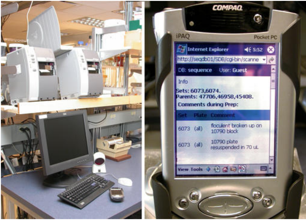
Figure 4. Barcodes are printed using networked Zebra printers (left). iPAQs provide a mobile interface into the LIMS (right).
