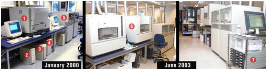
Figure 6. Sequencers: 1) MegaBACE 1000, 2) sequencer PC, 3) UPS, 4) sequencer power supply, 5) ABI 3700s, 6) ABI 3730XL and 7) x330 sequencer cluster.
